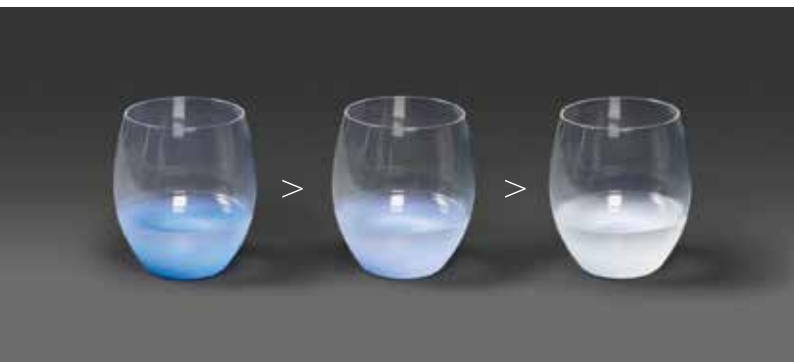
DEMONSTRATION OF THERMOCHROMIC WATER-BASED PAINT
